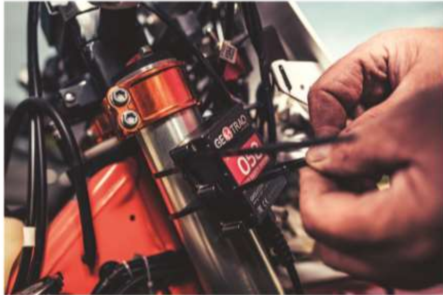
Installation of the GPS TRACKER on the suspension fork using cable ties.
